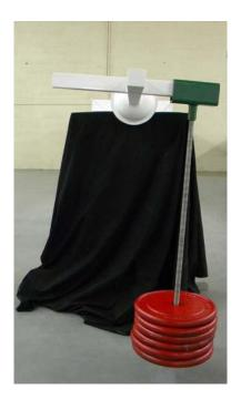
Twist Test Note: Weight is on extreme end of arm
